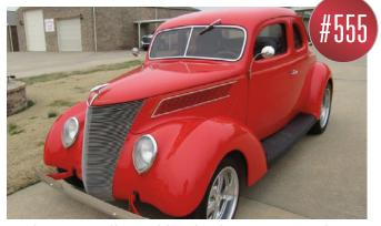
This is an all steel bodied car powered by an Edelbrock Fuel Injected 302 Ford V8 with a C4 transmission by TCI. Equipment includes power steering, front disc brakes, Vintage Air, Classic Instruments gauge package, electric
