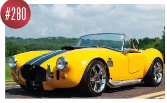
Car has never been raced; previous owner was a 75-year-old gentleman from Arizona. Previous owner stated no donor car parts were used during construction. Fully-chromed 454 CID big-block Chevy V-8, 10:1 compression and making 485 hp! GM high-performance heads yet runs on pump gas, Tremec six-speed manual transmission with 8.8-inch rear end and 4.10 gearing. Canary Yellow exterior with dual
