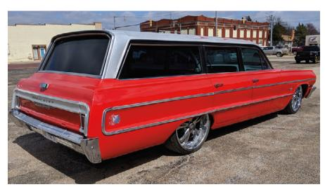
Custom wagon equipped with a LT1 350 V8 and 6 speed manual transmission from a 95 Chevy Camaro. Ride Tech air ride with electronic control in the dash, 20 inch Wheels with new tires, custom paint and new exhaust.
