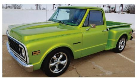
Less than 100 miles on a fresh overhaul 700 R4 automatic transmission, electronic fuel injection, 12 bolt rear end with 3:73 gears, House of Color Lime Gold Candy paint, Retro Sound radio and new gauge cluster. Power brakes, power steering and 18" Vision wheels.
