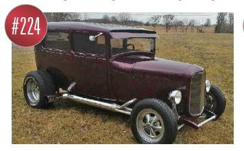
Hot Rod Chevy 350 V-8, 24 barrels, power steering. All steel body, 4 link 9" Ford rear end. Electric Suicide doors.
