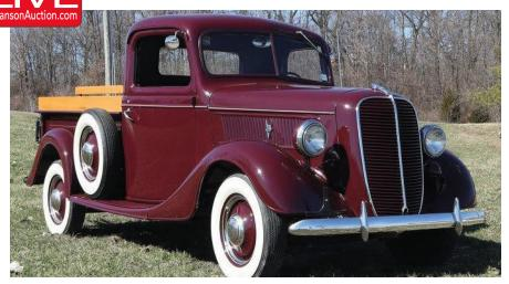
All steel body, steel fenders and running boards. New wood bed and wood slats, two tone vinyl interior, dual exhaust, Offenhauser intake and Offenhauser heads. 255 cu. In Mercury Flathead V8 with upgraded 4bbl carb.
