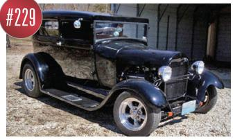
All steel body, American Racing wheels, coil over rear shocks with Ford 9" rear end 4-bar suspension. Front end 4-bar with 4" dropped I beam with front shocks. Front wheel disc brakes drum rear. Tinted back glass, custom gauges, AM/FM radio. New
