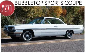
Debut year for third-generation Bonneville. One of 16,906 Bonneville two-door hardtops made in 1961. Correct optional 303 HP, BB-code 389 CID V-8 engine with 4 bbl carb, 10.25:1 compression and dual exhausts. 315 Pontiac Super HydraMatic automatic transmission. White exterior with Chocolate, Ivory and Copper-Beige seats in a Fawn interior (code 251).
