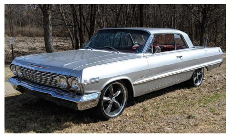
Complete Restoration with new 454 Big Block, 4 speed transmission, upgraded to Curry 9 inch Ford rear end, 4 wheel disc brakes. New paint and interior, new wheels and tires and new exhaust. This is a nice straight Impala SS that turns heads every time it is driven.
