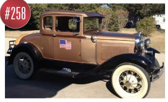
The Model A was the first Ford to use the standard set of driver controls with conventional clutch and brake pedals, throttle, and gearshift. The Model A's fuel tank was situated in the cowl, between the engine compartment's fire wall and the dash panel. It had a visual fuel gauge, and the fuel flowed to the carburetor by gravity. This great little coupe, has been fully restored in a great color combination, and runs perfectly.
