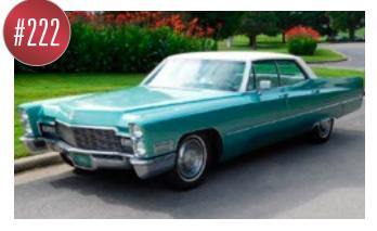
1968 was the first year for the powerful 472 cubic inch engine. In 1968 grilles had an insert with finer mesh and step down outer section which held the rectangular parking lights just a little higher than before. The most obvious change was an 8.5-inchlonger hood designed to accommodate recessed windshield wiper-washers, which now came with three speeds standard.
