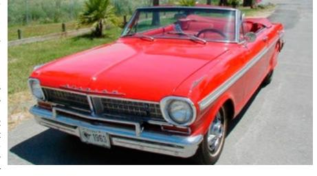
Pontiac. As with the concurrent Chevy II, Acadians were offered with 4 cylinder, 6 cylinder and V8 engines. There was a choice of transmission, depending upon the model and engine, 3 and 4 speed manual gearboxes or the 2 speed Powerglide automatic were available.
