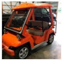
CT&T, maker of e Zone City & c Zone electric vehicles, is the largest Electric Vehicle Manufacturer in the world. C-ZONE has been acknowledged as the next generation golf car, leading the global golf car market through the CT&T 's exclusive high technology and ergonomic design. This multi purpose electric car has independent suspension, 4 wheel hydraulic brakes and heated seats. Ridged frame construction. Glass windshield and wipers. Sold on a bill of sale.
