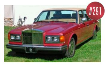
Rolls-Royce produced the Silver Spur from 1980 to 1989 as a long wheel base variant of the Silver Spirit. It was lower and wider than the outgoing Silver Shadow, but shared the same floorpan and 6.25 liter V8. New features included Girling automatic ride height control and Bosch injection from 1986 onwards. Limousine versions were available.
